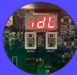
3-digit 7 segment display w/ 2 push buttons
